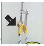
2. Attach the life raft lashing to the upper yellow thimble and secure the raft.
