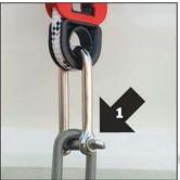
1. Use a shackle to secure the release to a fixed point on the deck or on the raft's cradle.
