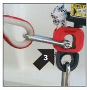
3. Connect the raft's painter line to the red weak link connector
